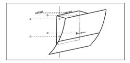
• Leave up the cooker hood and hang onto the wall bracket hook
