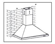
• Fix the lower chimney with 2 pcs of 4mm x 8mm screws.
