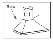
• Sliding the chimney to adjust the chimney height. When the height you required is reached, then fix 2 pcs of 4mm x 8mm screws onto the hole fixing with plate I as showed in below pictures.
