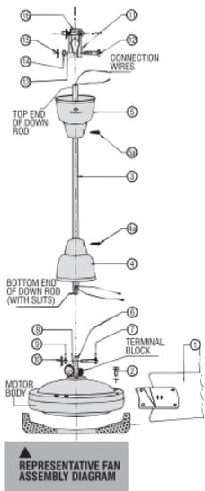
iii) Insert the bottom end of down rod (3) (with slits) on spindle (6) and insert bolt. (7) Place the spring washer (8) and fully tighten nut. (9) Insert the split pin (10) in the small hole on the bolt end and open the ends, so that it does not fall off. The assembly of bolt (7), spring washer (8), nut (9), split pin (10) is separately packed with the hanger assembly (11).
