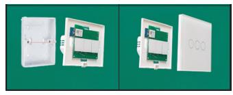
Fit the back of the smart switch in 3x3 inches electrical box
