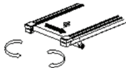
The adjustment for right deflection (diagram 3)
